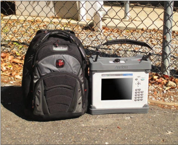
PIM Master MW82119A 40 Watts, Battery-operated
